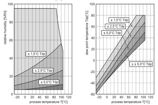
$\pm 1.5^{\circ}$ C ( $\pm 2.7^{\circ}$ F) at ambient temperature T < 25°C (77°F) a RH > 30%, for more details see graphs:
